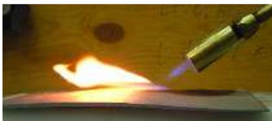
(top) Testing of the intumescent polyurea shows the coating expanding to slow the spread of fire and protect the substrate
